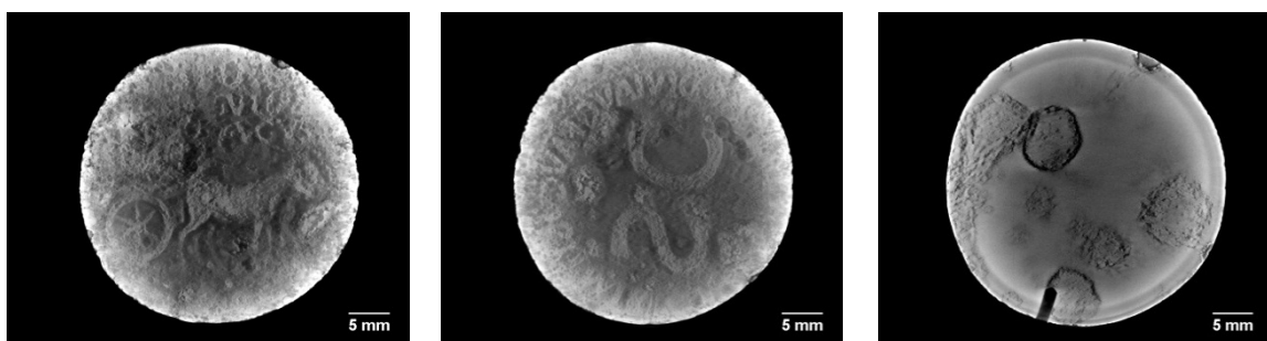
Figure 1 a-c: 3D- \mu XCT imaging a sestertius of Tiberius obverse (a), reverse (b) and inner part of the coin (c) with drill hole and showing depletion of zinc
