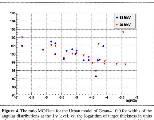
angular distributions at the 1/e level, vs. the logarithm of target thickness in units of radiation length. Results for all targets of electron scattering benchmark [24] are shown.
