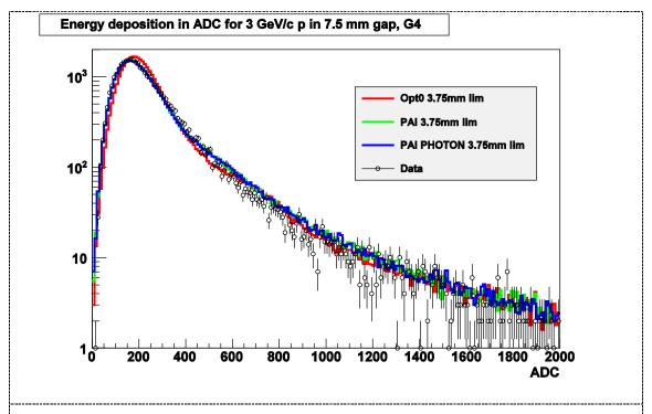
**Figure 3.** Proton energy deposition in gas gap in ADC counts: histogram – simulation (Opt0 means default model), open circles – data [22], [23]. Simulation was done with 1 mm cut, step limit is equal to half gap thickness 3.75 mm, beam momentum is 3 GeV/c, gas mixture Ne– $CO_2$ –N<sub>2</sub>; ADC scale for simulation was normalized on the PAI model peak position.
