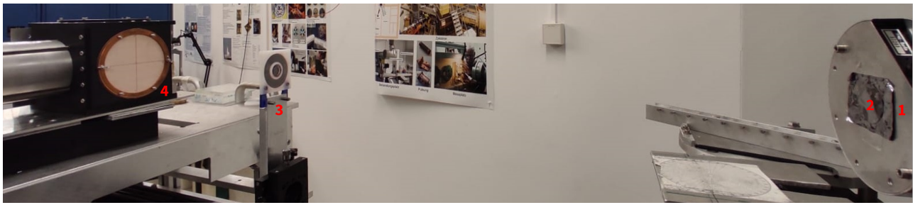
Figure 4: Nozzle setup: the beam travels from the end of the vacuum pipe (1) on the right toward the camera at the target position (4) on the left, undergoing double scattering from a thin aluminum foil (2) and a four-ring scatterer (3). A collimator aperture can be inserted at the position of the camera for the determination of the beam transmission using ionization chambers at both edges of the nozzle.
