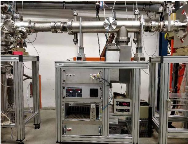
Figure 8: Beamline behind the Tandetron after installation of the Chopper.
