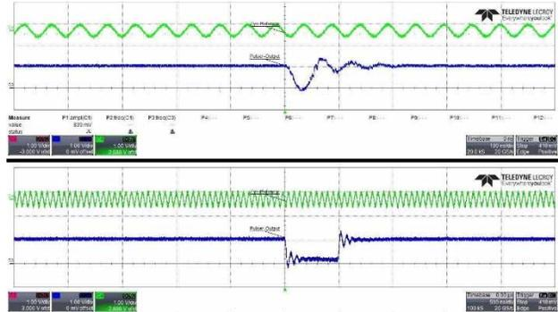
Figure 9: Above in blue is a 70 ns pulse and below in blue is a 500 ns pulse. The green signal is in both cases the cyclotron frequency of 19.3178 MHz.
