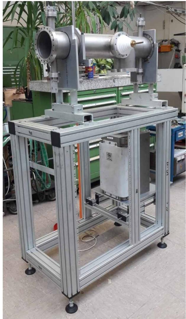
Figure 3: Vacuum chamber with the frame made of Item profiles.
