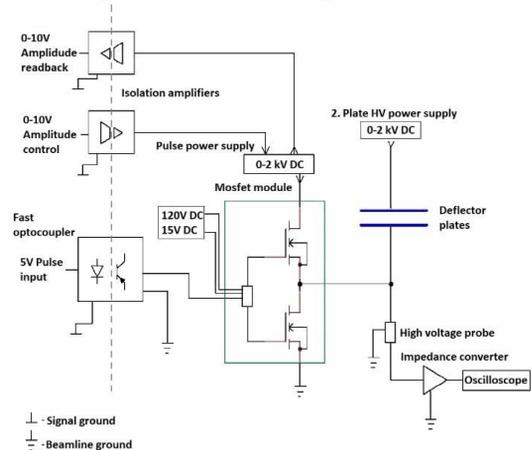
Figure 4: Operating principle of the fast Chopper.
