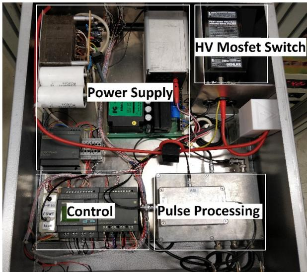
Figure 5: Processing and control electronics crate.
