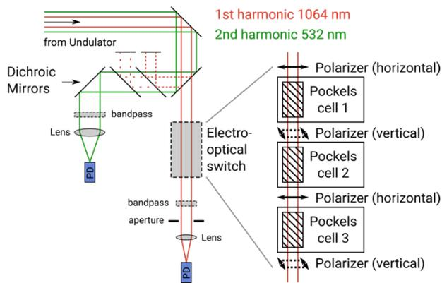
Figure 2: The signal detection setup is based on fast photodiodes. The powerful laser pulse has to be blocked for detection of the coherent signal by a series of three Pockels cells, because it has the same wavelength and direction. The coherent signal of the second harmonic can simply be singled out by optical filters.
