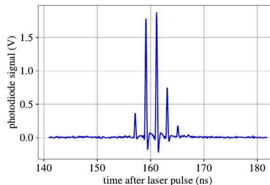
Figure 7: Sample of recorded signal; top: At  $t=0$  ns, the optical switch is still closed and only the attenuated laser shot is recorded. Shortly before the arrival of the coherent signal at 160 ns, the optical switch has been opened (grey trace); bottom: coherent signal after one revolution showing the electron bunches which interacted with the laser beam.
