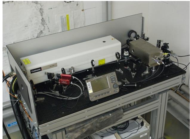
Figure 5: Optical table with the laser setup in the storage ring bunker.
