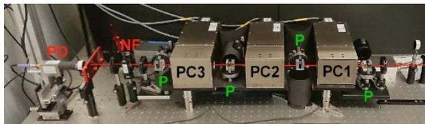
Figure 3: Signal detection setup at the undulator beamline: Three Pockels cells (PC) are placed between crossed polarizers (P). Additional filters (NF) can be placed in front of the photodiode detector (PD).
