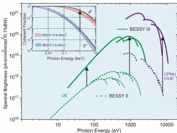
Figure 3: Spectral brilliance and coherent flux of BESSY III compared to BESSY II.
