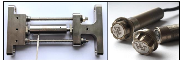
Figure 6: Encapsulated piezo in the housing frame (left), and separating bolt before and after trigger (right).
