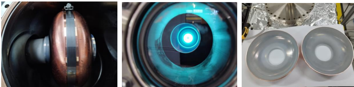
Figure 8: The copper half-cell cavity with magnetron at iris (left), magnetron as seen from the iris (center), coated two half-cell cavities (right).
