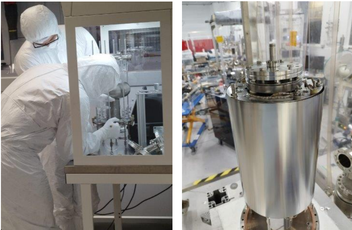
Figure 6: Preparation of cavity assembly in iso-4 cabinet (left) and fully assembled Nb cavity for deposition (right).
