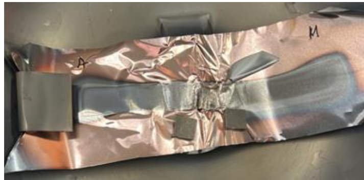
Figure 9: Slotted two half-cell cavities and witness samples attached with copper foil.
