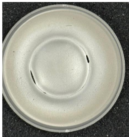
Figure 14: \text{Nb}_3\text{Sn} target after the cavity coating. Along the race-track, areas where erosion has completely consumed the target are visible.
