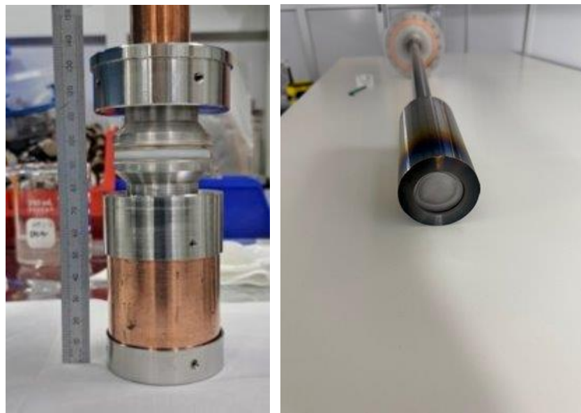
Figure 7: The 2-inch planar magnetron for coating internal surface of 1.3 GHz SRF cavity designed and build at UKRI/STFC.
