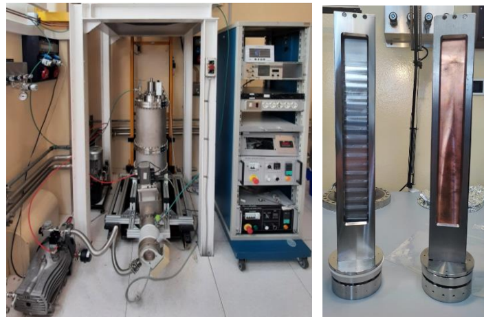
Figure 3: From left to right: scheme of deposition system, picture of the deposition system at INFN, Al and Cu Rectangular Magnetron mounted.
