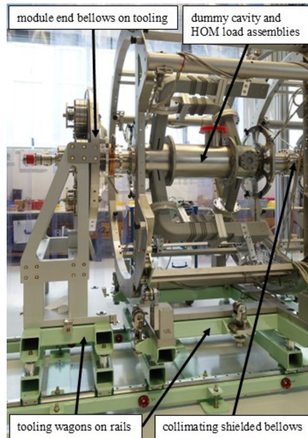
Figure 3: Completed cold string assembly in the spaceframe.
