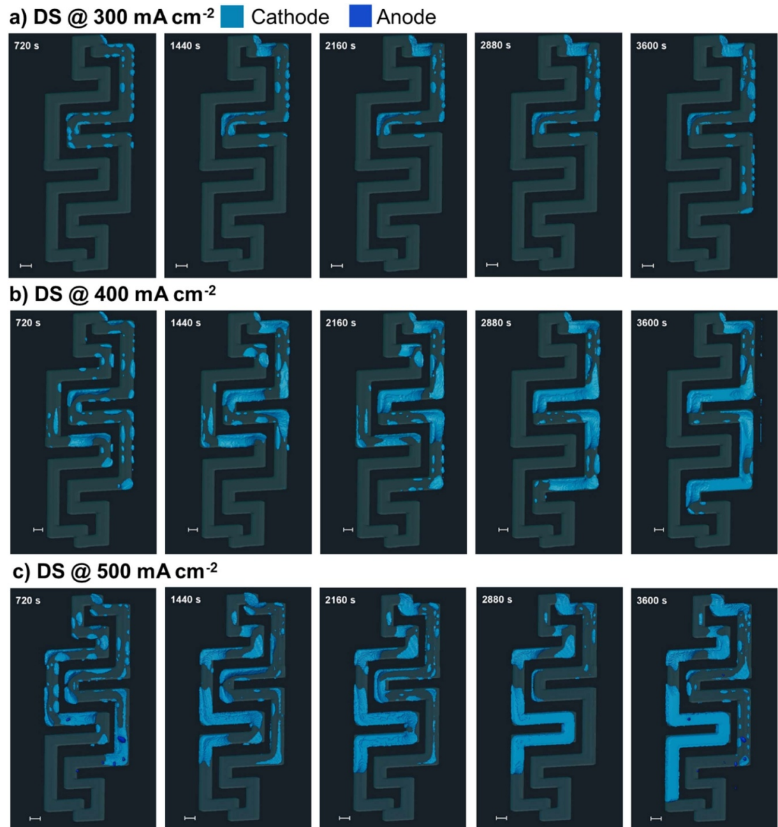
Figure 7. Water evolution in the DS flow fields during the (a) 300 mA cm -2 , (b) 400 mA cm -2 and (c) 500 mA cm -2 galvanostatic holds. Cathode water is shown by light blue and anode water shown in dark blue, although little water in the anode was observed in any of the current holds. The scale bar represents 1 mm in all images.
