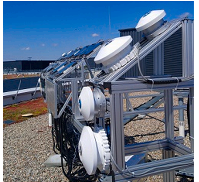
Fig. 1. PVcomB-HZB outdoor testing facility showing the two pairs of spectrometers for optimum and vertical angles facing south.
