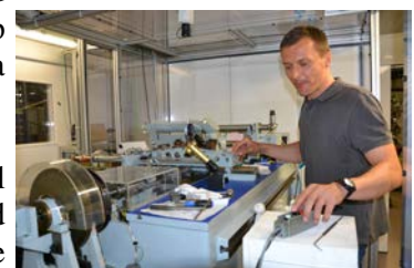
This machine is used to create the sawteeth. A diamond is used to etch tiny grooves into gold coated silicon substrates.
