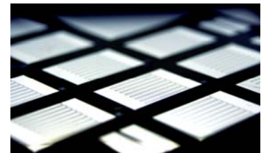
Comb-shaped, interdigitated metal contacts on the side facing away from the sun of back-contact silicon heterojunction solar cells. Pictured are several test cells on a single silicon wafer. Image source: HZB
