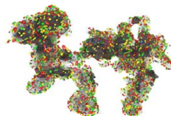
Depiction of catalyst nanoparticles: The particles (coloured) adhere to a substrate (grey). They are imaged by electron tomography. For imaging, the data are processed using novel algorithms.
