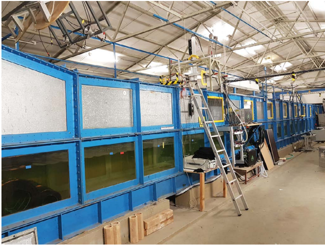
Fig. 4: Wind-wave tunnel facility at the University of Hamburg. Photo: Martin Gade.
