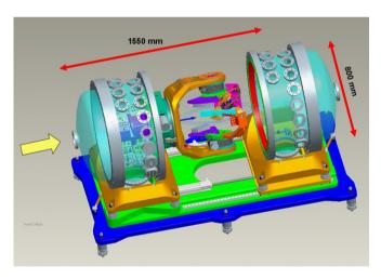
Fig. 2. Schematic setup of the new reflectometer.
