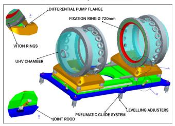
Fig. 8. The UHV-chamber for the reflectometer with the adjustable stand.
