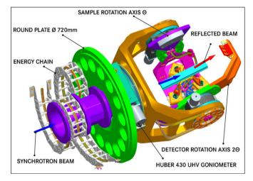
Fig. 7. Sample azimuthal rotation.
