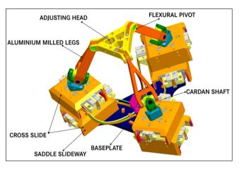
Fig. 3. The tripod unit for sample adjustment in six degrees of freedom.
