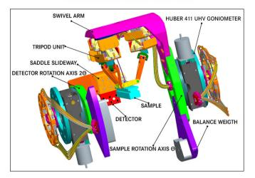
Fig. 6. Sample and detector rotation.
