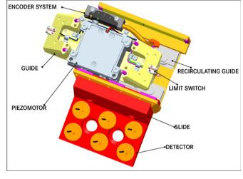
Fig. 5. The detector arm translation stage.
