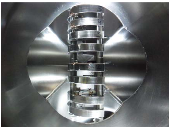
Figure 10. Transfer system. “magazine” for 11 samples.
