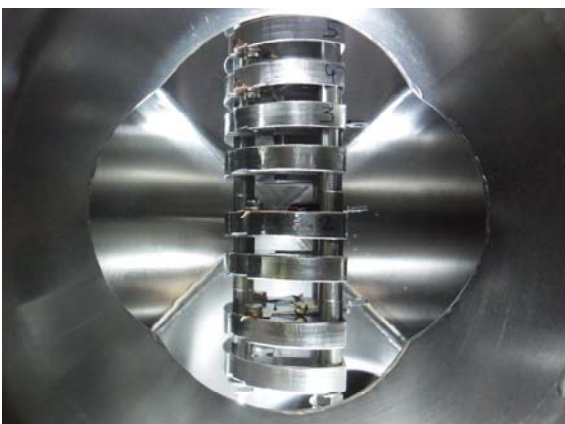
Figure 10. Transfer system. “magazine” for 11 samples.
