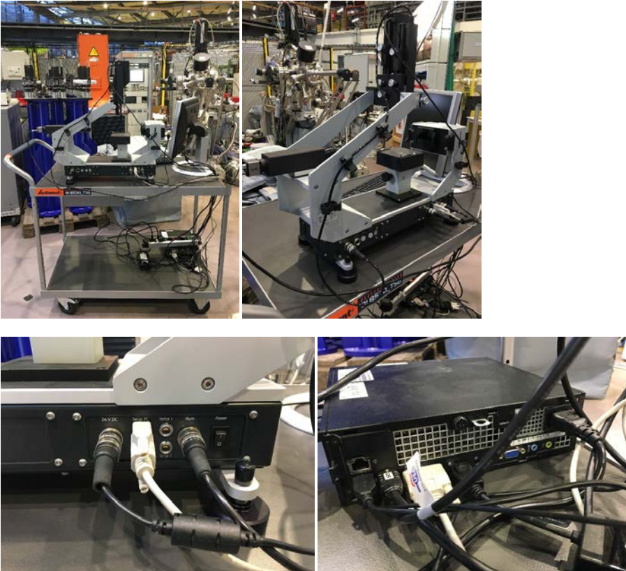
Figure 3: Installation of cables of the DSA25
