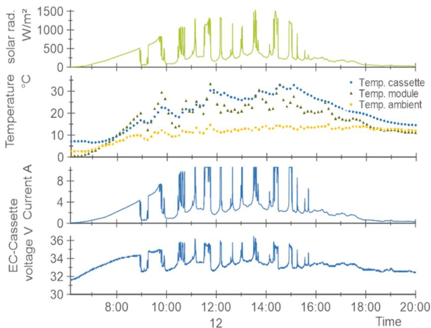
**Figure 6.** Slowly moving clouds: diurnal variation of irradiance, temperature and electrical power reference values of one HJT PV module from ENEL directly coupled to a 21-cell PEM electrolyser stack (12<sup>th</sup> May 2020).
