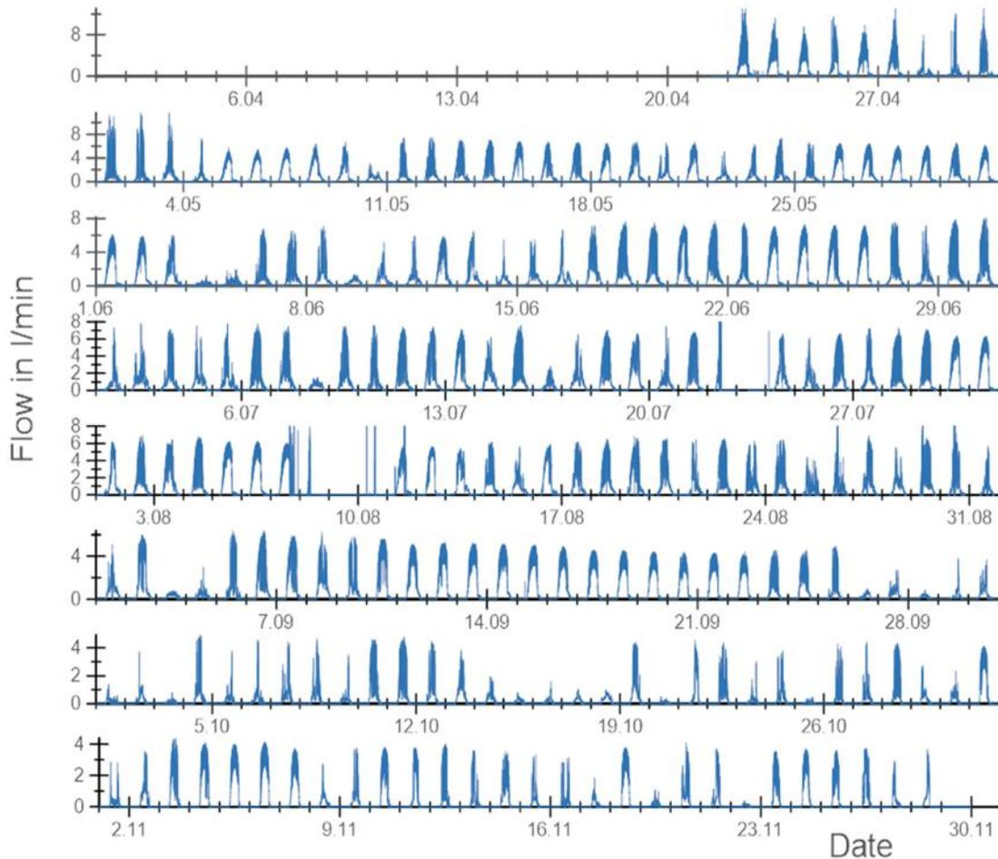
**Figure 8.** Daily variation of hydrogen generation during the operation in outdoor conditions in Jülich, Germany for the period from April to November 2020 measured in the whole demonstrator.
