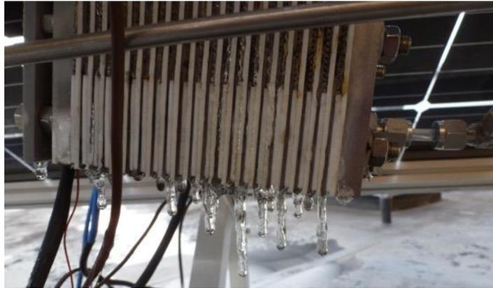
**Figure 14.** Frozen electrolyser stack during winter operation (30<sup>th</sup> November 2020).
