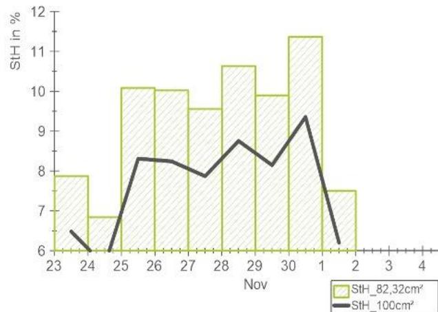
**Figure 17:** Solar to hydrogen (StH) efficiency in UU integrated system during November 2020.
