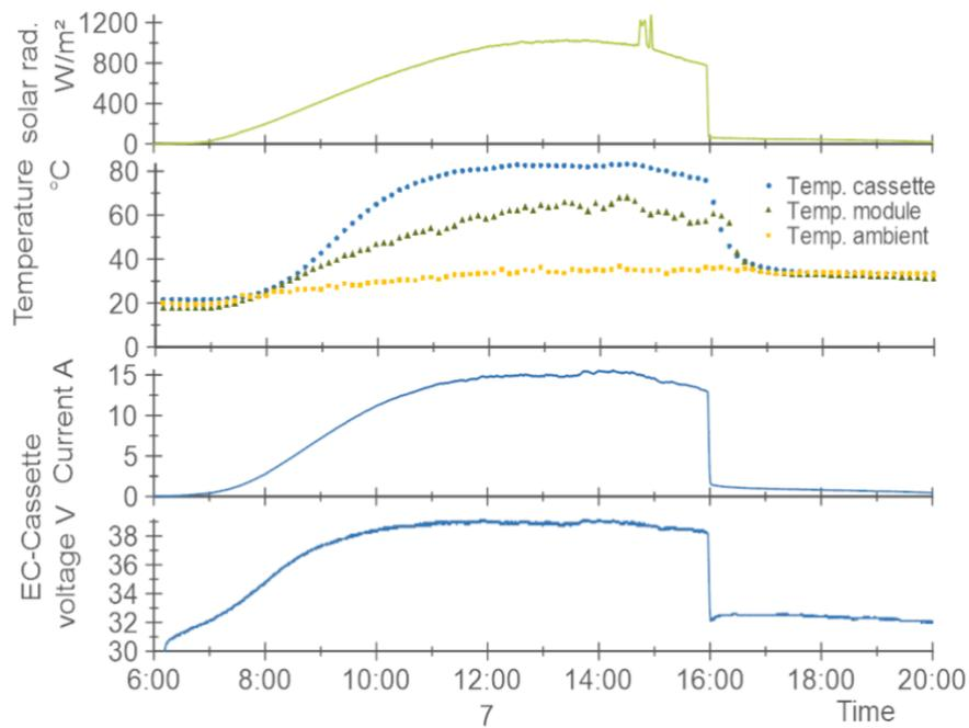
**Figure 5.** Sunny warm day: diurnal variation of irradiance, temperature and electrical power reference values for operation of two HJT PV modules from ENEL directly coupled to a 21-cell PEM electrolyser stack (7<sup>th</sup> August 2020).
