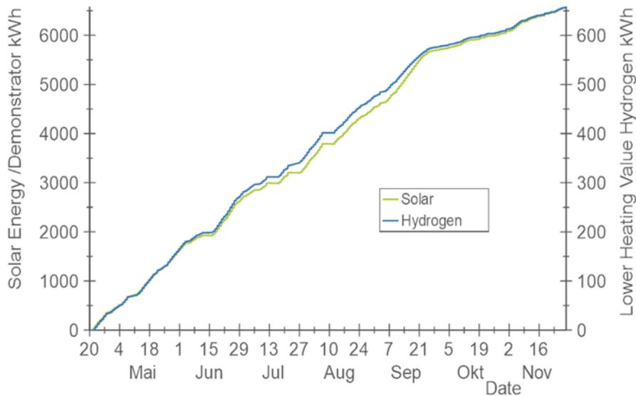
**Figure 9.** Time evolution of the incident solar energy and stored energy (hydrogen lower heating value basis) over the operation period from 20<sup>th</sup> April to 2<sup>nd</sup> November 2020 of the entire 10 m<sup>2</sup> direct solar hydrogen generation demonstrator.
