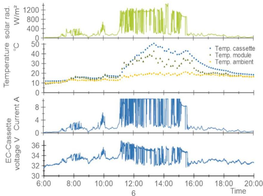
**Figure 7.** Fast moving clouds irradiance, temperature and electrical power reference values for operation of a xxx PV module directly coupled to a 21-cell PEM electrolyser (6<sup>th</sup> June 2020).
