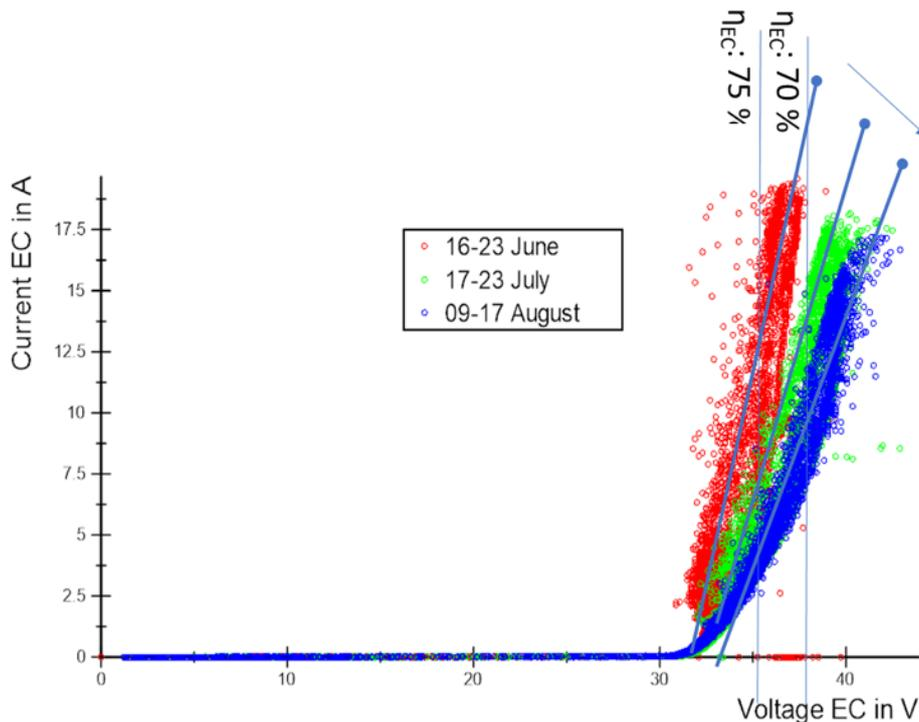
**Figure 13.** Degradation of the a 21-cell stack with standard loading electrolysis cells that remained in service (directly connected to two HJT PV modules in parallel) up to and after the end of the project.
