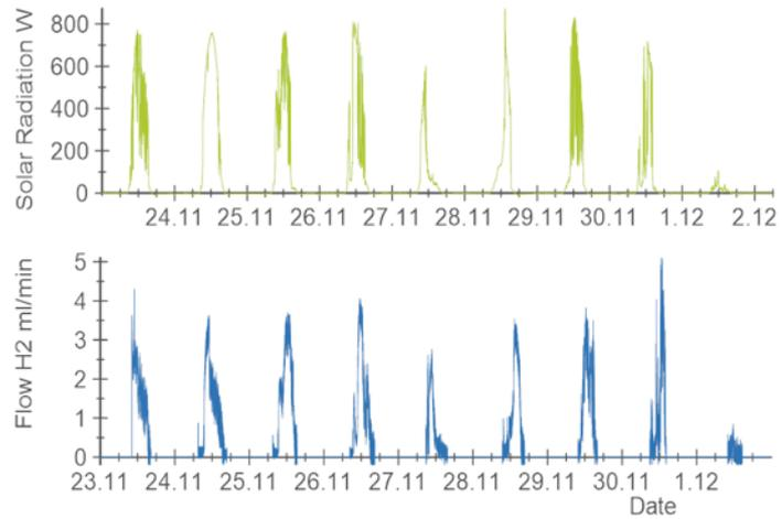
**Figure 16:** Solar radiation and hydrogen generation in the CuInGaSe photovoltaic integrated alkaline electrolyser showing operation from 23<sup>rd</sup> November to 2<sup>nd</sup> December 2020.
