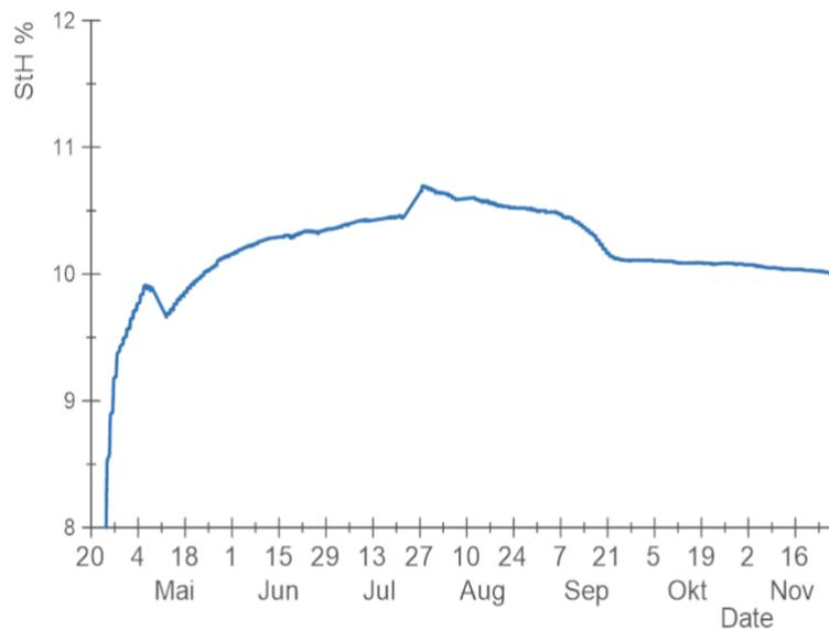
**Figure 11.** Solar to hydrogen efficiency over the operation time from April to November 2020 of the entire 10 m<sup>2</sup> demonstrator plant.
