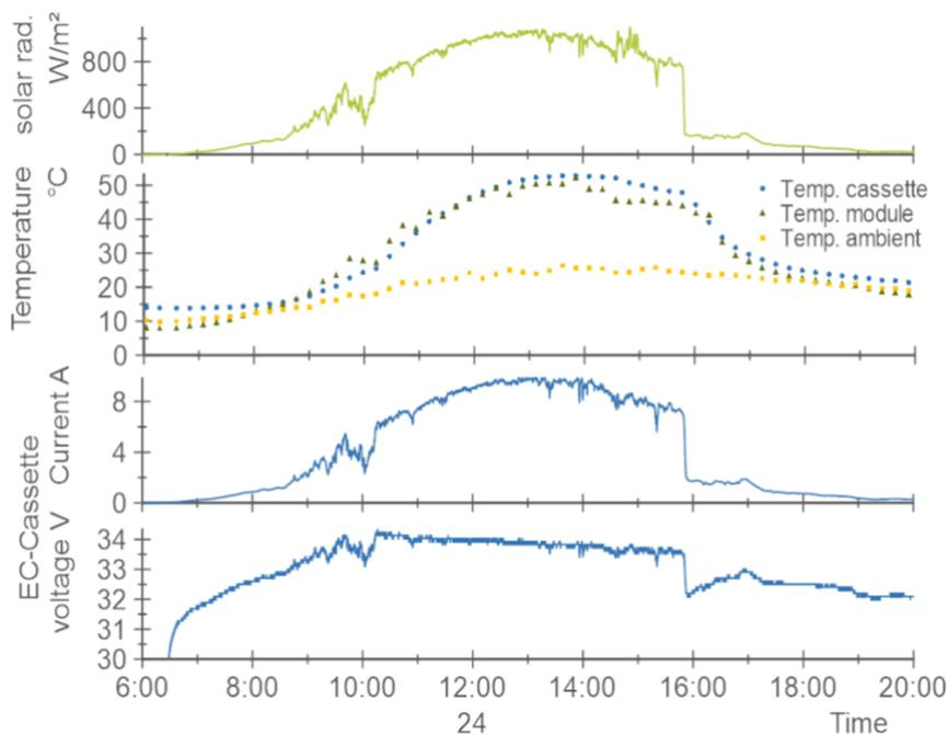
**Figure 4.** Sunny cold day: diurnal variation of irradiance, temperature and electrical power reference values for operation of one HJT PV module from EGP directly coupled to a 21-cell PEM electrolyser stack (24<sup>th</sup> April 2020).
