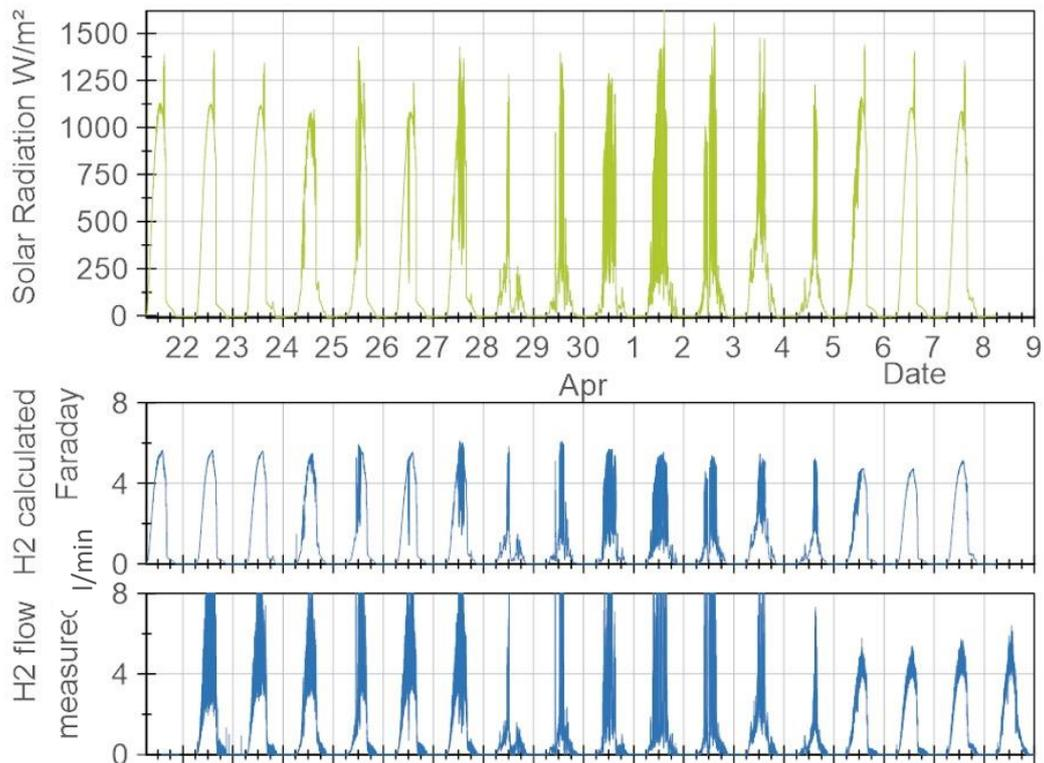
**Figure 2.** Measured solar radiation, hydrogen production calculated from measured electrolyser currents by Faradaic law and measured hydrogen flow [l/min] for operation between 21<sup>st</sup> April to 9<sup>th</sup> May 2020 with 8.25 m<sup>2</sup> PV total area installed. One additional 2 m<sup>2</sup> SHJ PV panel was installed later.
