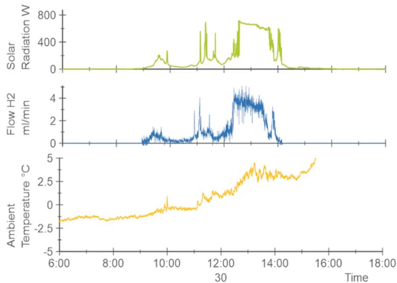
**Figure 18:** Diurnal variation of solar radiation and ambient temperature and the resultant hydrogen flow rate illustrating low temperature operation of the CIGS integrated alkaline electrolysis prototype on 30<sup>th</sup> November 2020.
