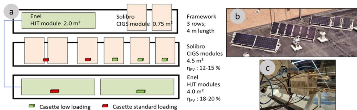
**Figure 1.** (a) Schematic showing the different PV module + electrolyser (EC) sets. (b) Aerial view of the final setup of the 10 m<sup>2</sup> demonstrator plant, photographed in July 2020. The two modules on the top right-hand side are not connected to electrolysers. (c) Photograph showing the PEM electrolyser directly mounted onto the back of one of the silicon heterojunction (HJT) PV modules in the so-called cassette design.
