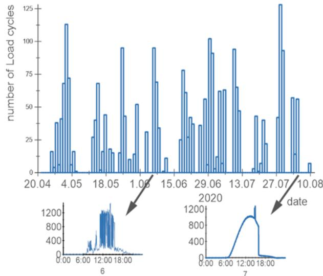
**Figure 12.** The effect of fluctuations in incident irradiance on the dynamic operation (quantified by number of load cycles per day) of the PEM electrolyzers driven by the photovoltaic modules.
