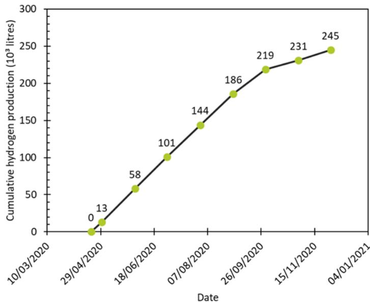
**Figure 10.** Cumulative volume of hydrogen generated over operating duration from 20<sup>th</sup> April to 2<sup>nd</sup> November 2020 of the entire 10 m<sup>2</sup> direct solar hydrogen generation demonstrator. The cumulative hydrogen yield from this period was 735kWh.
