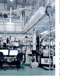
In EMIL a large variety of deposition instruments are connected to analytics with light from BESSYII via a fully automatised UHV-transfer backbone.
