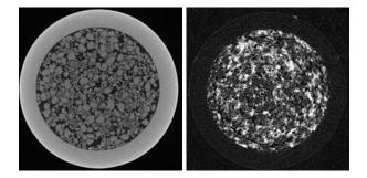
Fig. 1 Tomographic slices of a compacted silica sample with water measured by (left) X-rays (pixel size: 12  $\mu$ m; exposure time: 2.5 s; 1000 projections) and (right) cold neutrons (pixel size: 13.5  $\mu$ m; exposure time: 120 s; 500 projections). The diameter of the AI container is 10 mm. (courtesy of Dr. D. Penumadu, University of Tennessee).
