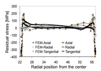
Figure 2: Residual stress distribution measured along the radius compared to simulation results
