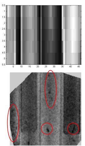
Fig. 2 Dark-field (USANS) radiography of cylindrical AlSi samples taken in the double crystall diffracto-meter V12a (top), and corresponding measurement [3] with a grating interferometer at the radiography instrument CONRAD (bottom) Note that the grey scale is inverse as compared to the upper image.
