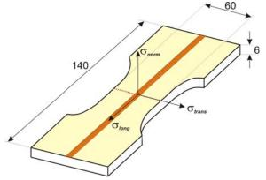
Figure 1: Shape of the used samples
