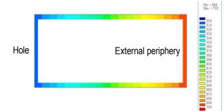
Figure 1: Distribution of the heat transfer coefficients on the half disc
