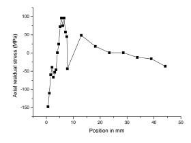
Figure 2. Axial Residual stress along Fe/weld interface
