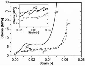
Figure 1: Example for twinning stress reduction of a polished sample due to repeated mechanical deformation. Average twinning stresses decreased from around 12 MPa to 1.5 MPa after four compressions. Inset shows serreated flow of stress-strain curve.
