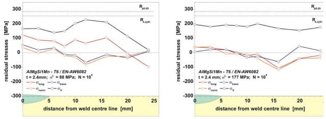
Figure 4: Residual stress distributions 2.4 mm below the surface after cyclic loading (R = 0.1) with load amplitude of 40 MPa (left) and 80 MPa (right).
