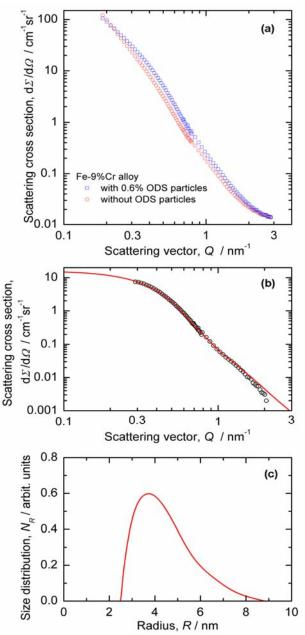
Fig. 1: (a) Measured SANS intensities of Fe-9%Cr model alloys with 0.6% and without ODS nanoparticles, (b) difference scattering curve (symbols) and data fit (line), (c) calculated size distribution, number density per radius interval,  $N_{R_1}$  of ODS nanoparticles.
