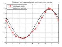
Figure 2: Measured and approximated (by sin-function) wall thickness for tube 5 over circumference.
