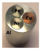
different samples (Fe, Ni, Co) inside were adjusted. A vertical slit (width = 1mm) in front of the sample, perpendicular to the incident beam, was shifted in 23 steps, and for each step the total scattering curve was measured.
