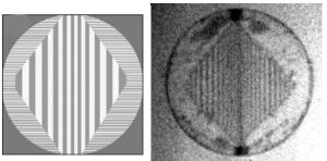
Fig. 2 Schematic representation of the magnetic domains in the investigated SiFe plate (left side) and the corresponding dark-field image visualizing domain walls
