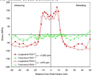
Figure 2: Influence of tool rotational speeds on the residual stress distributions
