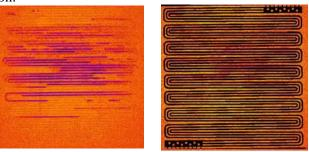
Fig.3: Masking out the channels for better analyses of water volumes under the ribs.
