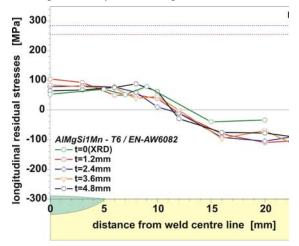
Figure 3: Longitudinal residual stress distributions in different depths in comparison the surface values (XRD).
