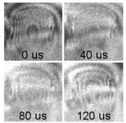
Fig.2. Stroboscopic images of magnetic field measured with the spin-polarized neutron beam and an analyzer installed in front of neutron counting detector with microchannel plates. Continuous sequence of frames, each 2  $\mu$ s in duration, was acquired for the entire 333  $\mu$ s-long cycle. Only 4 frames out of the entire sequence are shown. The legend indicates the time delay from the beginning of the AC cycle. The amplitude of the AC current was 10 A.
