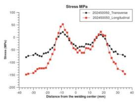
Fig.2 Residual stress in the Al2024 specimen. The 0 value in the abscissa axis represents the center of the welding.
