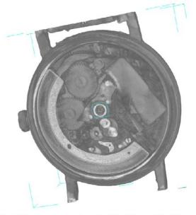
Fig.2 The same watch as in Fig.1 but with 180µm resolution with the V12c set up.
