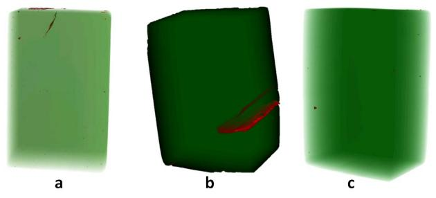
Figure 1: Exemplarily three dimensional reconstructions of defects found in three samples of the new grown  $Ni_{49.7}Mn_{29.3}Ga_{21.0}$  single crystal ingot. Pores and surface cracks can be identified in (a), two large cracks that reach in a sample and are close to combine are shown in (b), and a small pore is shown in (c). All samples shown here have dimensions of approximately  $6 \times 4 \times 3 \text{ mm}^3$ .
