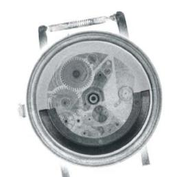
Fig.1 Reconstruction of an old watch with 85µm resolution with PONTO, size of the watch ~ 40mm
