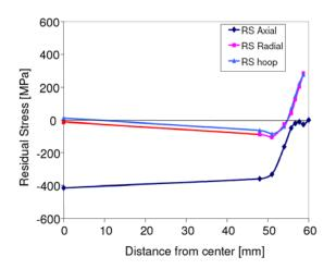
Figure 2: Axial, hoop and radial residual stresses plotted against the distance from the central plane of the bar (drawn with a die angle of 20°)
