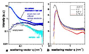
Fig. 2: Double log plot of the scattering intensity I vs. the scattering vector q. (a) empty beam, test cell without carbon, carbon electrode only and carbon electrode in test cell with "zero matched" water. (b) Scattering for differently charged EDLC electrodes.
