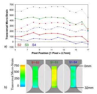
**Fig. 2:** Transversal strain obtained by Bragg Edge Imaging a) along specimen height b) spatially resolved
