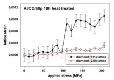
Figure 3: The Al/CD/60p ht 10h with different strains in diamond (111) lattice compared to (220).
