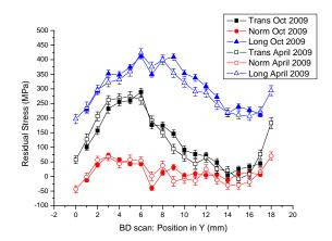
Figure 3. Weld transverse, longitudinal and normal along a line through thickness
