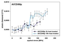
Figure 1: Diamond lattice strains in Al/CD/60p after 3h and 10h heat treatment.
