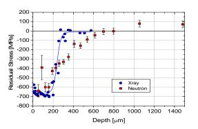
Figure 1. Residual stress profile of a shot peened ferritic steel sample as determined by neutron diffraction on E3 (red symbols). For comparison the averaged results form a round robin campaign using X-Ray diffraction [3] is also given (blue).
