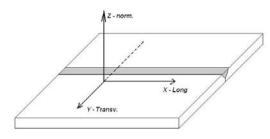
Fig.1 - Geometry of the samples measured direction in the butt joint sample.
