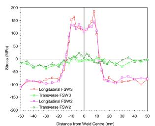
Figure 1: Influence of tool traversal speeds on the residual stress distributions
