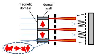
Fig. 1 Schematic representation of the contrast formation by magnetic domain walls in a grating interferometer set-up for neutron imaging.
