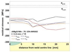
Figure 2: Residual stress distributions 2.4 mm below the surface in the as-welded state.
