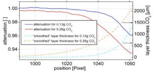
*Fig.2:* Evaluation of the radiographies show the normalized attenuation caused by deposited  $CO_2$  (for two amounts of  $CO_2$ ) within the sample along the vertical middle axis of the sample. The evaluated zone is at the cold side of the sample holder. In addition the calculated layer thickness of  $CO_2$  is depicted.
