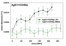
Figure 2: Diamond lattice strains in AgSi11/CD/60p with two different diamond particle types (JR1/MBD4).
