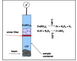
Fig. 1: Experimental set-up
