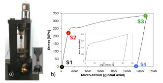
**Fig. 1:** a) Portable Loading system (and specimen with rosette gauge b) recorded Stress-Strain of tensile test (inset: Torsion)
