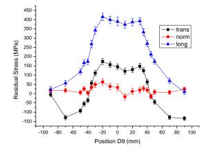
Figure 2. Weld transverse, longitudinal and normal 9mm below the surface of the plate.
