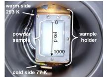
*Fig.1:* The experimental setup consists of the sample holder for a vacuum chamber with feed throughs for  $LN_2$ ,  $CO_2$  and electrics. The black arrow represents the evaluated zone.
