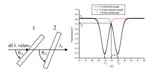
Fig 3. The principle of the extraction of the wanted wavelength  $\lambda_i$  from the initial polychromatic neutron beam. Transmissions of single crystals are given by their mosaicities (red and blue lines). The resulting transmission of the crystal pair is shown with open symbols.
