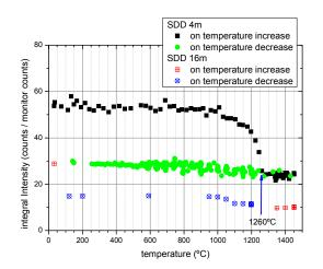
Fig. 1: Integral intensities scattered to small angles, predominantly by the lamellar  $Cr_{23}C_{6}$ -type carbides.
