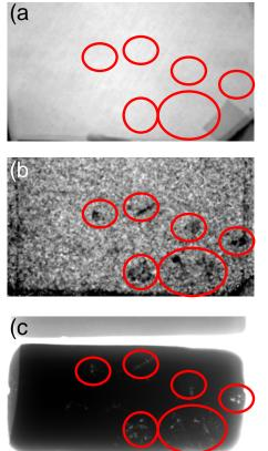
Fig. 1 Neutron attenuation, dark-field and x-ray image of BiSn sheet [2]
