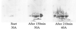
Fig.1: Temporal development of the water management in a PEM fuel cell by means of in-situ neutron radiography
