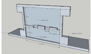
Fig.1 Drawing (slice plane) of the used aluminium diffusion-cell for the experiment
