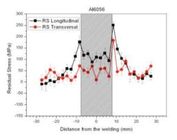
Fig.3 Residual stress in the Al6056 specimen
