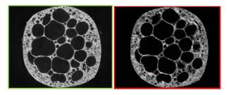
Fig. 2 Tomographic slices of borated aluminum foam by (left) X-rays (pixel size: 12  $\mu$ m; exposure time: 2.5 s; 1000 projections) and (right) cold neutrons (pixel size: 13.5  $\mu$ m; exposure time: 120 s; 500 projections). The foam size is 6 mm in the horizontal direction.
