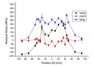
Figure 1. Weld transverse, longitudinal and normal 2mm below the surface of the plate.
