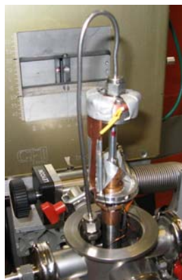
Figure 1: Al-Pressure cell (0-200 bar) mounted at the V1 instrument. The inner diameter of the cell is 4 mm.
