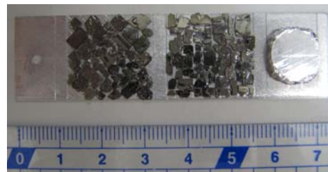
Fig. 1 Photo of the sample mosaic. CeCoIn 5 with [110] axis vertical (left), with [100] axis vertical (centre) and an Nb crystal for initial alignment of the field with the neutron beam. All samples were mounted on one plate and we changed between them by changing height of the dilution stick in the magnet.
