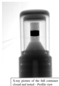
Fig. 1: Radiogram of the sample enclosed inside the double-wall certified Al-capsule developed by ITU.
