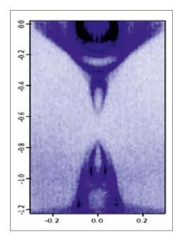
The experiment at the U125-2PGM undulator beamline of BESSY II shows bands with opposite curvature, so-called Fermi arcs. © HZB
