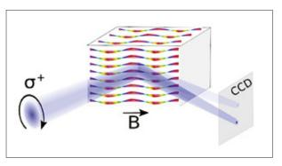
The picture reflects the main effect: A circular polarized soft-X-ray beam scatters off a crystal that exhibits a helical or conical magnetic order. This leads to two scattered beams of different intensity. © F. Radu/HZB
