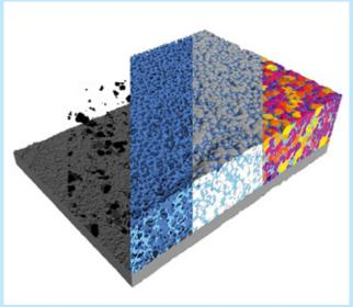
X-ray tomography of a battery cathode, virtually disassembled into its components. © M. Osenberg, I. Manke/HZB/Binder/KIT
