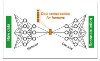
With the help of special neural networks, raw data can first be compressed and then reconstructed in such a way that it can be interpreted by scientists. © G. Hartmann et al.
