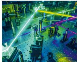
In the femtosecond laser laboratory, charge transport in semiconductors can be studied with terahertz and microwave spectroscopy. For this purpose, laser pulses first generate charge carriers in the material, which then absorb long-wave radiation (terahertz or microwaves) proportional to their mobility.
