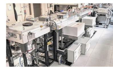
The cluster facility operated at HZB allows to produce large-area perovskite/ silicon tandem solar cells. This facility, the only one of its kind in the world, helps to develop new industry-related processes, materials and solar cells. © B. Stannowski/HZB
