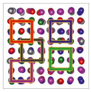
The Cantor alloy under study consists of chromium (grey), manganese (pink), iron (red), cobalt (blue), and nickel (green). X-ray methods allow to probe each individual component in an element-specific way.
