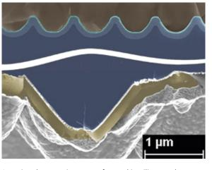
Scanning electron microscopy of perovskite silicon tandem cells in cross-section with nanotexture and back-reflector layer (golden). © P. Tockhorn/HZB
