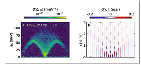
The data from neutron scattering (left) provide information about absorbed energies in reciprocal space. With the new evaluation, it has been possible to obtain statements about new magnetic states and their temporal development in real space (right). The colours blue and red indicate the two opposite spin directions. © HZB
