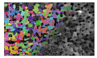
Electron microscope image of a silicon sample with nanocrystallites of different orientation (coloured), pores (black) and the pore network recognised by the image processing software (white grid lines). ©: D. Kojda/HZB
