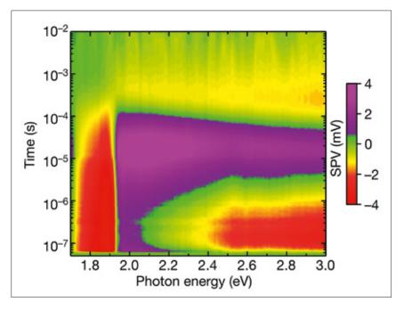
Contour plot of  $\text{EH-Cu}_2O$ . The photovoltages are plotted as a function of photon energy (x-axis) and time (y-axis). Positive SPV signals (purple regions above 1.9 eV) correspond to the relaxation of holes trapped on {111} facets, whereas negative SPV signals (red regions) correspond to the relaxation of electrons trapped on {001} facets. © T. Dittrich/HZB
