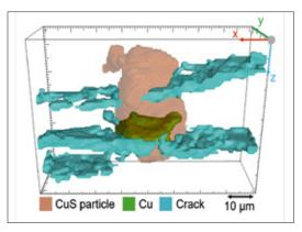
3D reconstruction of the formation of a copper crystallite in a copper sulfide particle (CuS) during the discharge of a lithium CuS solid-state battery. The volume expansion can lead to the formation of cracks (blue).
