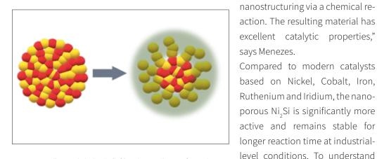
Crystalline nickel silicide (left) is chemically transformed into nanostructured material with excellent catalytic properties for the electrolytic splitting of water and the production of valuable nitrile compounds.
