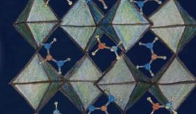
Triple Cation Triple Halide Perovskite  $[\text{Cs}_{0.05}(\text{MA}_{0.05}\text{FA}_{0.95})_{0.95}]\text{Pb}(\text{I}_{0.95}\text{Br}_{0.05}\text{Cl}_{0.0x})_3$
