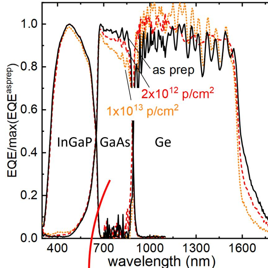
Radiation Damage in the GaAs middle subcell
