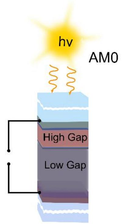
Radiation damage in the low gap bottom subcell
