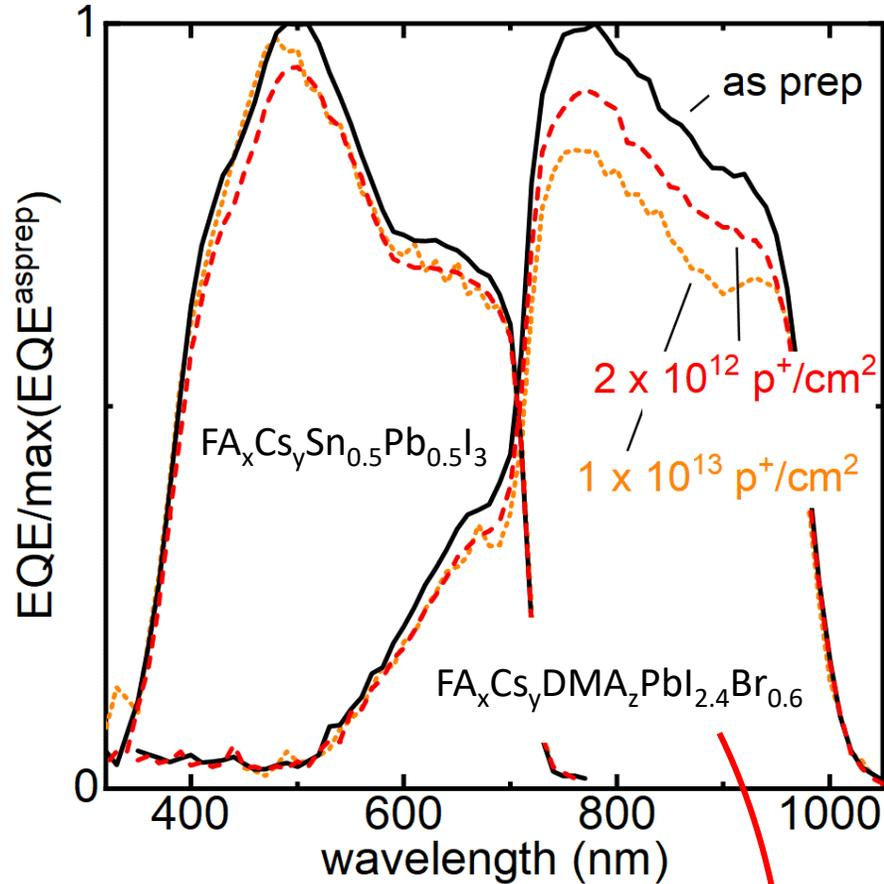
Radiation damage in the low gap bottom subcell
