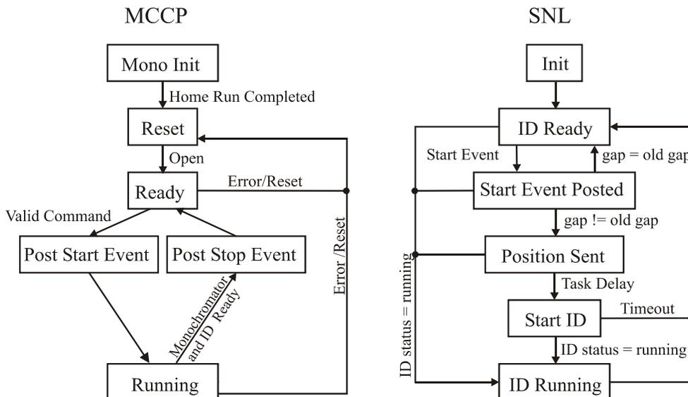
Figure 2: State transition diagrams of the Monochromator Control Program MCCP (left) and State Notation Language SNL Program (right).
