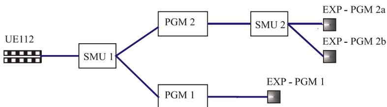
Figure 1: Schematic of the BESSY Beamline at the UE112 undulator. The low photon energy monochromator at U112-PGM2 has been designed to meet the requirements for high flux and high resolution at a photon energy range from 5eV to 250eV [3] that complements the U112 - PGM1 beamline with a photon energy range from 15 eV to 600eV
