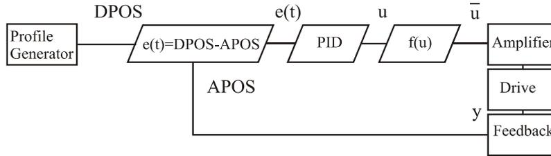
Figure 5: Structure of the user programmed feedback loop for PMAC2-VME. Amplifier, drive and feedback can be described by a Hammerstein model [12]. The error of the system is determined by the difference of the desired position (DPOS) and actual position (APOS). A linear PID Filter / Feedforward control calculates  $u$  which is mapped to  $\bar{u}$ . PMAC outputs  $\bar{u}$  to the to the amplifier box of the drive.
