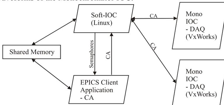
Figure 3: Communication and concept of Soft IOC for determination of quadrature errors.
