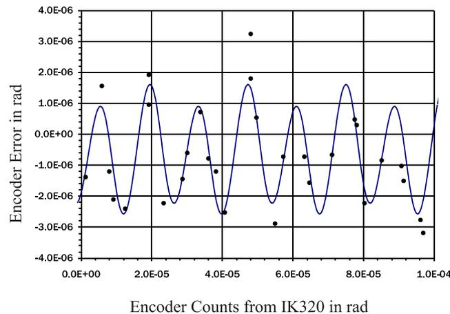
Figure 4: Experimental verification of the quadrature error. Dots are determined from Hydrogen absorption spectra.
