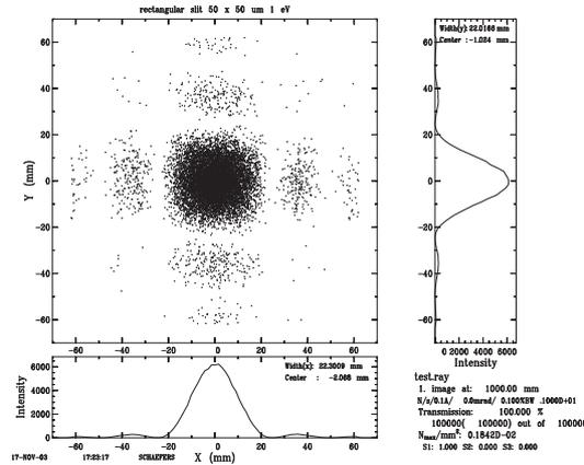
Fig. 2.12. Fraunhofer diffraction pattern on a rectangular slit
