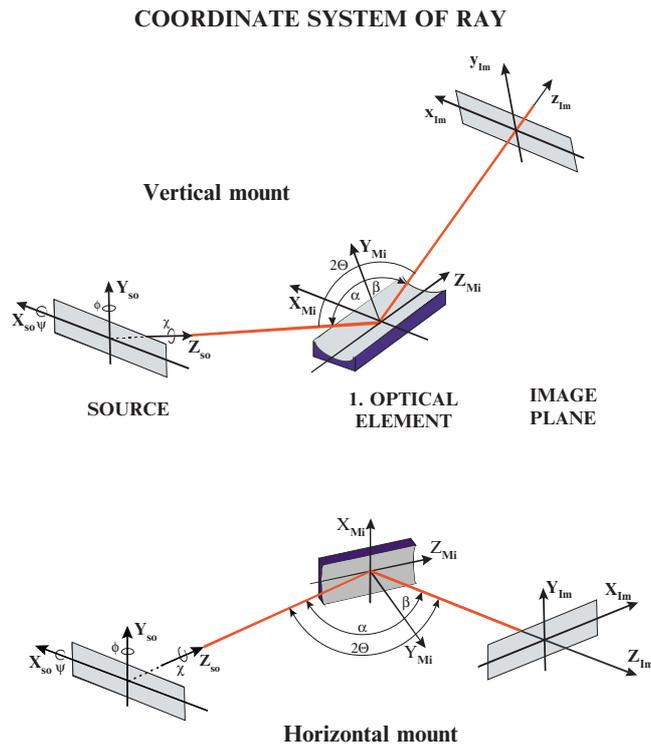
**Fig. 2.6.** Coordinate system (right-handed screw) and angles used in RAY. (*Top*) Vertical deviation (upwards (downwards)) mount (azimuthal angle  $\chi = 0^\circ$  ( $180^\circ$ )). (*Bottom*) Horizontal deviation (to the right (left)) (azimuthal angle  $\chi = 90^\circ$  ( $270^\circ$ )). The optical element is always in the  $X_M$ - $Z_M$ -plane
