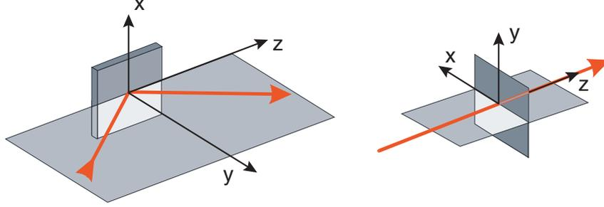
**Fig. 2.7.** Coordinate systems used in RAY. For optical elements (*left*) the coordinate system is fixed to the optical surface ( $X$ - $Z$  plane). Transmission elements, screens and image planes (*right*) are in the  $X$ - $Y$  plane, the  $x$ -axis is in the horizontal plane. The red line is the light beam
