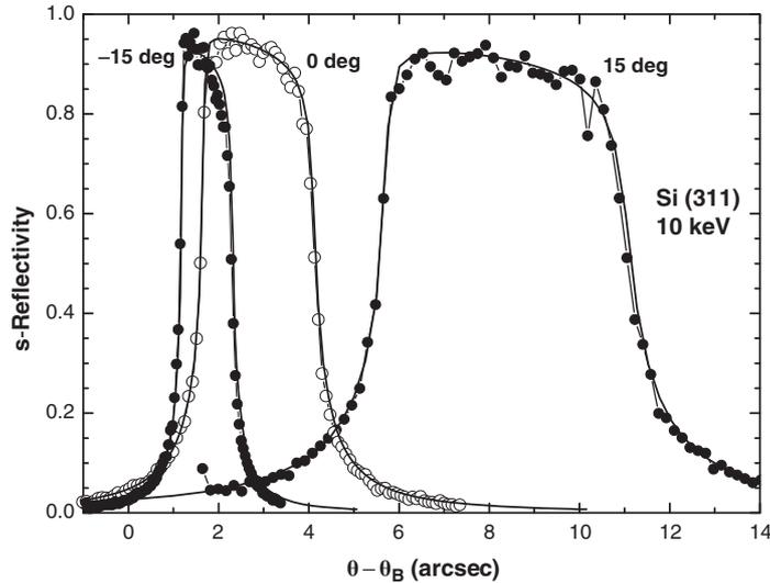
**Fig. 2.14.** Rocking curves of Si(311) crystal with asymmetric cut ( $15^\circ$  and  $-15^\circ$ ) and symmetric cut ( $0^\circ$ ) for  $\sigma$ -polarisation at a photon energy of 10 keV
