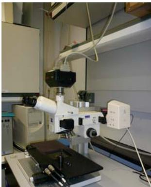
Left: Fluorescence microscope with spot illumination
