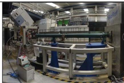
The reflectometer V18 BioRef is a versatile time-of-flight instrument dedicated to the investigation of soft matter thin films and interfacial structures at solid-air and solid-liquid interfaces. The chopper system allows for tailoring the resolution of the instrument to the requirements of the specific measurement as well as for kinetic studies.
