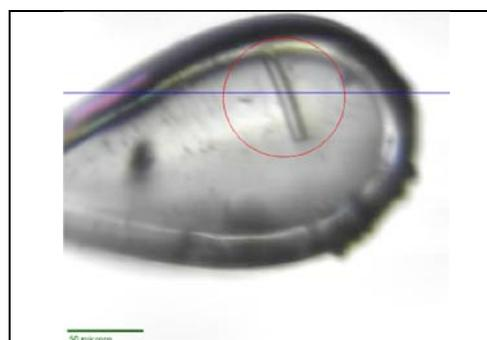
11  $\mu\text{m}$  crystal within a 50  $\mu\text{m}$  X-ray beam
