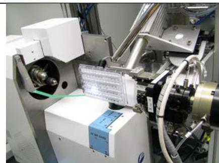
BL14.1 is a state-of-the-art MX beamline and currently the most modern and efficient MX beamline in Germany. It is energy-tunable within the range from 5 keV (2.5 Å) to 16.5 keV (0.75 Å). BL14.1 is equipped with an automatic sample handling robot (CATS). The MD2 microdiffractometer, which is equipped with a mini-kappa goniometer and on-axis sample zoom-microscope, enables the visualization and 3D-centring of crystals at a micrometer scale in the X-ray beam.
