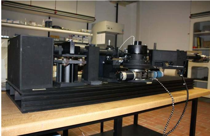
Dynamic light scattering instrument, manufactured by ALV
