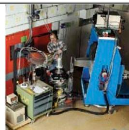
The diffractometer V1 with variable incident wavelength is installed at the curved neutron guide NL 1A. It is equipped with a high-resolution area detector. The design of the instrument is dedicated for experiments with biological membranes, polymers, micro-emulsions, micelles and other partly oriented systems. The high spatial resolution of the detector is appropriate for studying reflections from biological single crystals and magnetic satellite reflections.
