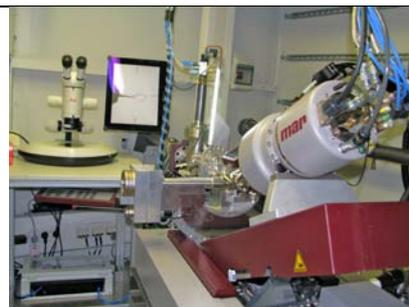
BL14.3 is a fixed energy beamline which is operated at an energy of 13.8 keV (0.89 Å). It can be used for *de novo* structure solution using anomalous phasing methods such as SAD utilizing heavy atoms like Pt, Hg, Au, Se and others. BL14.3 offers a unique experimental set-up to improve the diffraction properties of protein crystals. It is equipped with a HC1c dehydration setup, which can be used to improve the diffraction quality of crystals by controlled dehydration.
