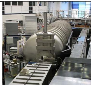
The very small-angle scattering instrument V16 (VSANS) serves for the analysis of mesoscopic structures, usually diluted in a buffer liquid. As the method is sensitive to variations in the scattering length density even pores can be investigated. Contrast variation techniques, namely deuteration of sections of the molecules to be investigated are crucial to obtain a maximum of information.
