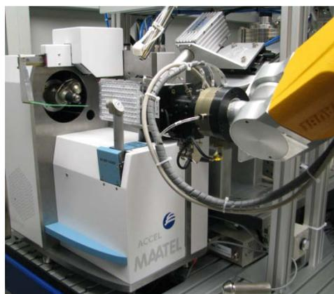
Figure 2 A crystallization plate with samples ready for X-ray analysis
