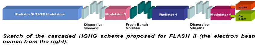
Figure 5.1: Design FLASH II - HGHG Undulator Section [4]
