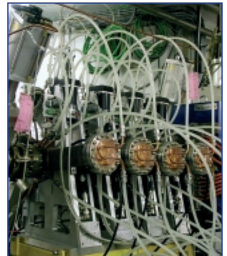
Fig. 2: Photo of the four 1.5 GHz Landau cavities installed upstream of the BAM-WLS.
