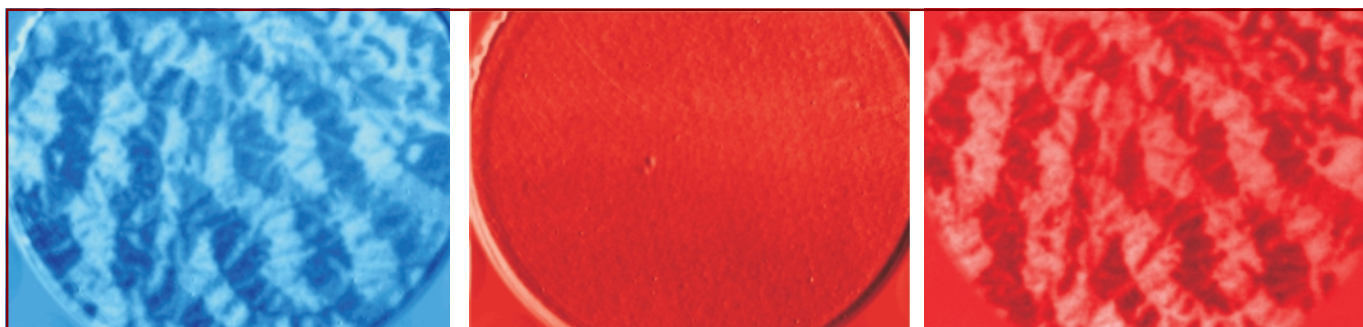
Fig. 2 shows magnetic contrast of \text{Co}_2\text{Cr}_{0.6}\text{Fe}_{0.4}\text{Al} by photoelectron emission microscopy. A ferromagnetic coupling between Iron and Cobalt is seen by the similar magnetic contrast of the micrometer-sized domains measured at the corresponding absorption edges. At the Chromium Edge no contrast of magnetic origin is observed.
