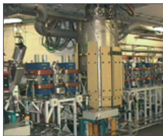
Fig. 4: Photo of the 6 T wavelength shifter, formerly operated at BESSY I, that replaced the 4 T device.
