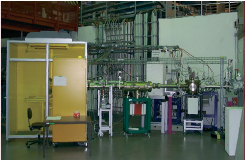
Fig. 4: EUV beam line at BESSY: pre-mirror chamber on the right, multi layer mirror chamber in the middle, clean room hutch with exposure station on the left.
