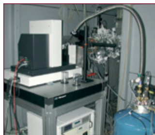
Fig. 1: Experimental setup for protein crystal diffraction at BAMline (Protein Structure Factory).
