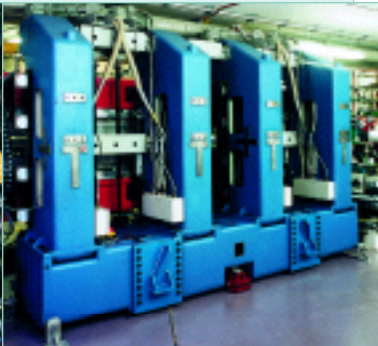
Undulator to enhance the radiation brilliance
