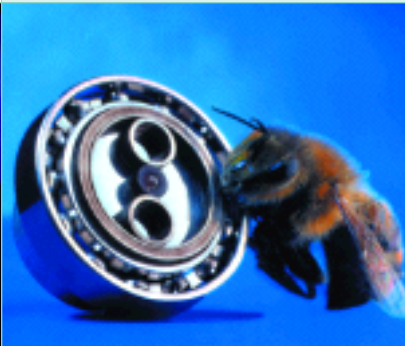
Microgear manufactured by using synchrotron radiation
