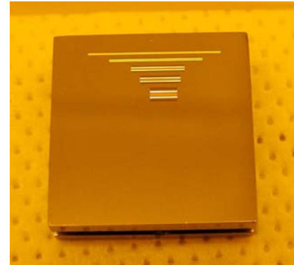
Figure 3. Lenses for energy 24.34 keV, 16.11 keV, 8.98 keV, 7.11 keV, 4.04 keV. Focus distance is 310 centimeters. Last zone size is 300 nanometers.
