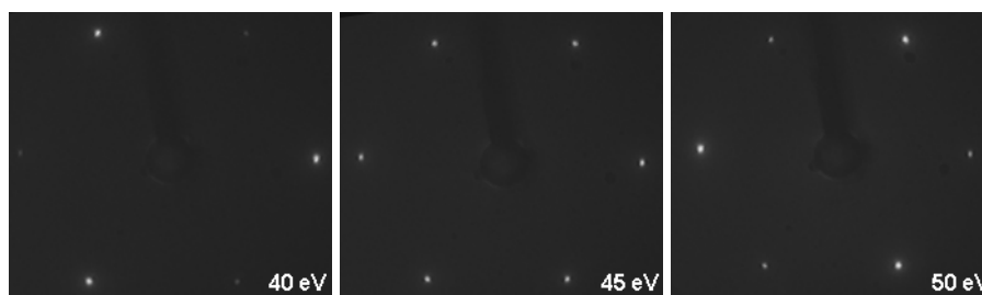
Figure 3: LEED patterns of Si(111)-CH 3 . The (1x1) symmetry is consistent with a methyl-termination.
