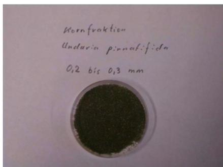
Fig. 3: Particle fraction of *Undaria pinnatifida* between 0.2 and 0.3 mm
