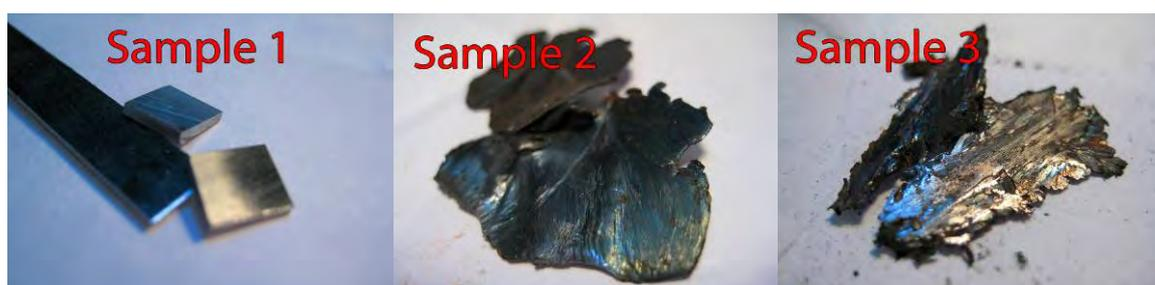
**Figure 1. Sample1 – initial state of steel, Sample2 – scaled structure formed on the wheel surface during friction, Sample3 – part of wheel that adhered to the brake block**
