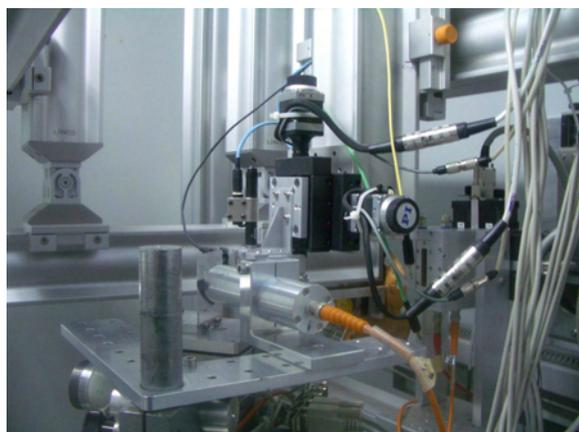
Fig. 5: Measuring station (sample, detector (Si-PIN photodiode), synchrotron beam line KMC-2)
