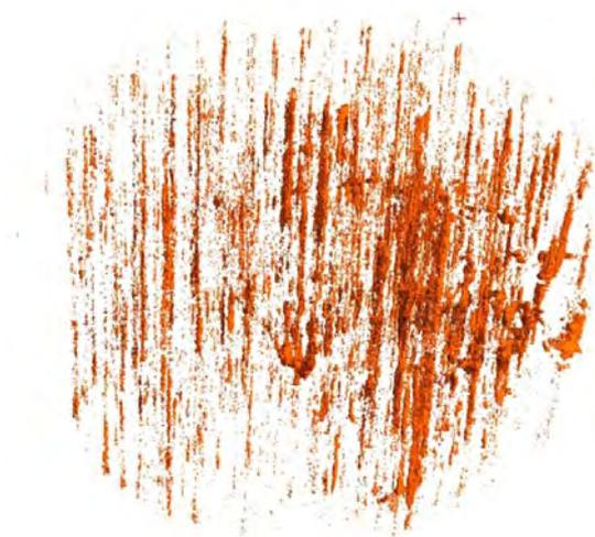
Figure 9: Visualization of fatigue cracks along the fibre surfaces of the LCF sample without matrix and fibres. The scattering plane of the analysing crystal was perpendicular to the fibre direction.
