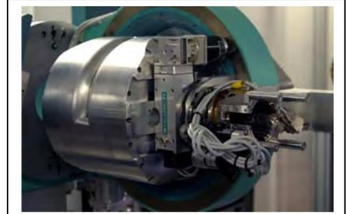
Fig. 1: The new compact 50 kOe superconducting magnet at MAGS, mounted to the Euler cradle of the diffractometer together with the cryostat holder (right hand side).
