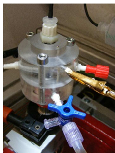
Fig.: Cell for electrochemical mass spectrometry
